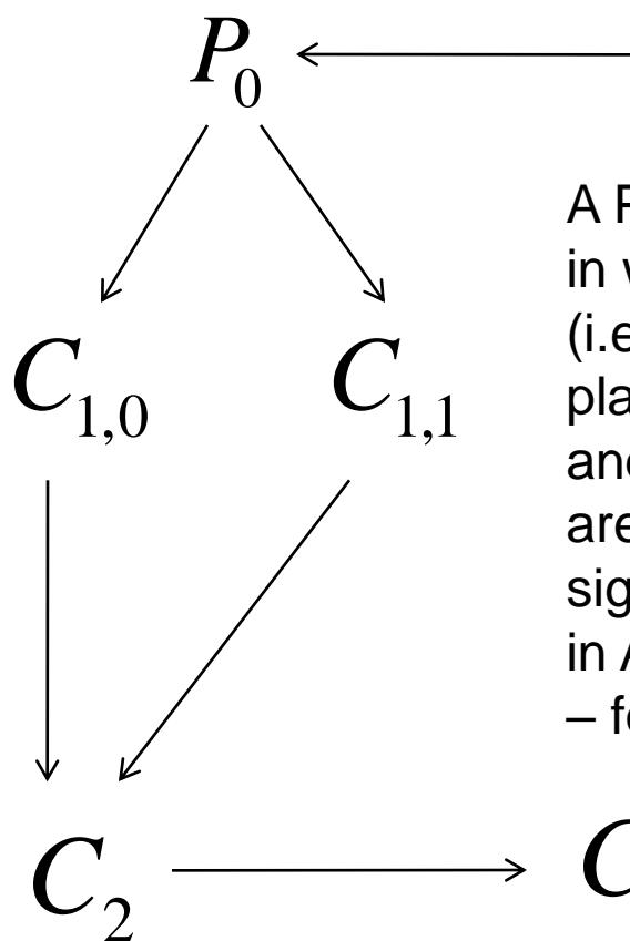
A Petri net is a directed bipartite graph, in which the nodes represent transitions (i.e. discrete events that may occur, signified by bars), places (i.e. conditions, signified by circles), and directed arcs (that describe which places are pre- and/or postconditions for which transitions, signified by arrows). Petri nets were invented in August 1939 by Carl Adam Petri – at the age of 13 – for the purpose of describing chemical processes.
